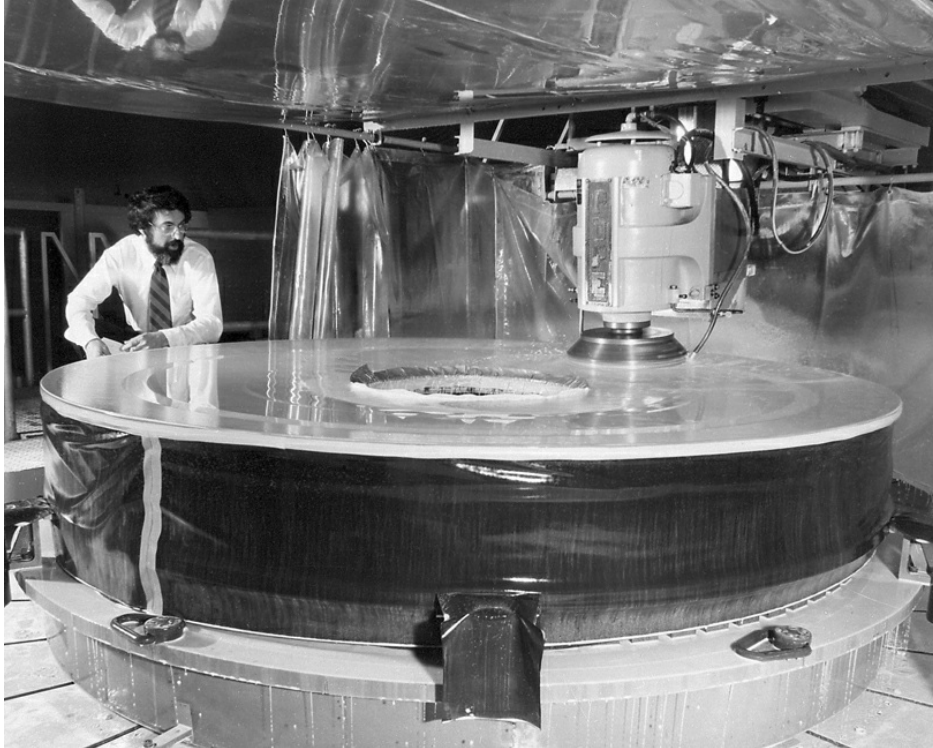
The Hubble telescope's eight-foot-diameter primary mirror being polished at the Perkin-Elmer Corporation's top-secret facility in Danbury, Connecticut. An overlooked measurement error on the mirror amounting to one-fiftieth the thickness of a human hair managed to render most of the images beamed down from Hubble fuzzy and almost wholly useless.
