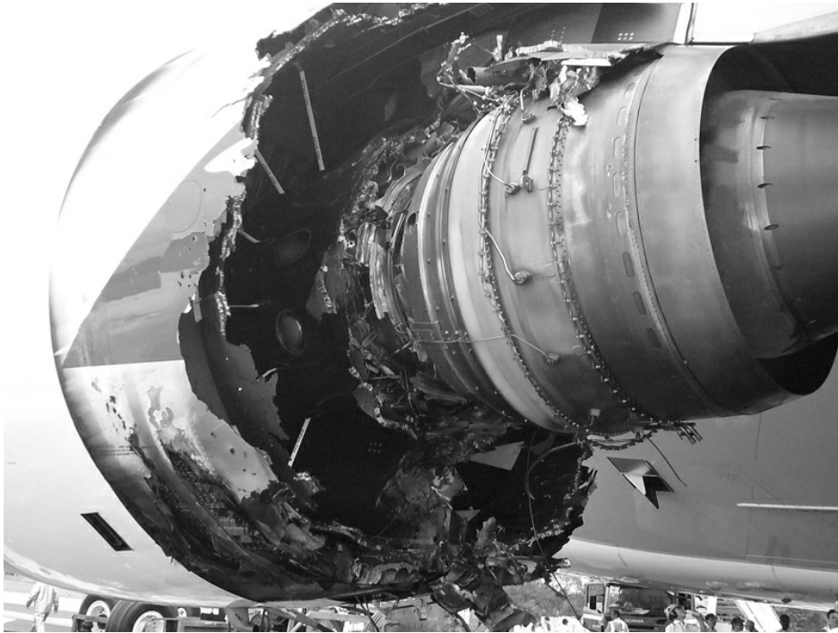
The wholly destroyed Rolls-Royce Trent number two engine after the safe landing in Singapore of Qantas Flight 32 following an “uncontained rotor failure” inside the engine a mile high over Indonesia.
