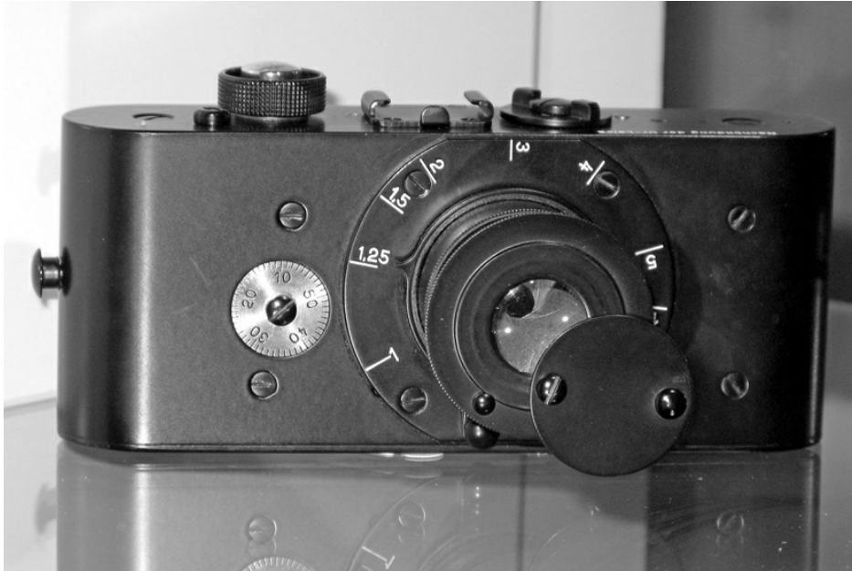
The prototype Ur-Leica, fashioned in 1913 by the Leitz employee Oskar Barnack. It was small, light, with a near-silent shutter, and a 24 × 36 mm film format.
