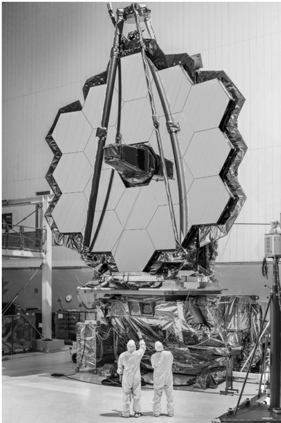
The main mirror for the James Webb Space Telescope. At more than twenty-four feet in diameter, it will, from its location a million miles from Earth, vastly increase our ability to peer into the very edge of the universe, and at the time the universe was forming. It is due to be launched in 2019.
