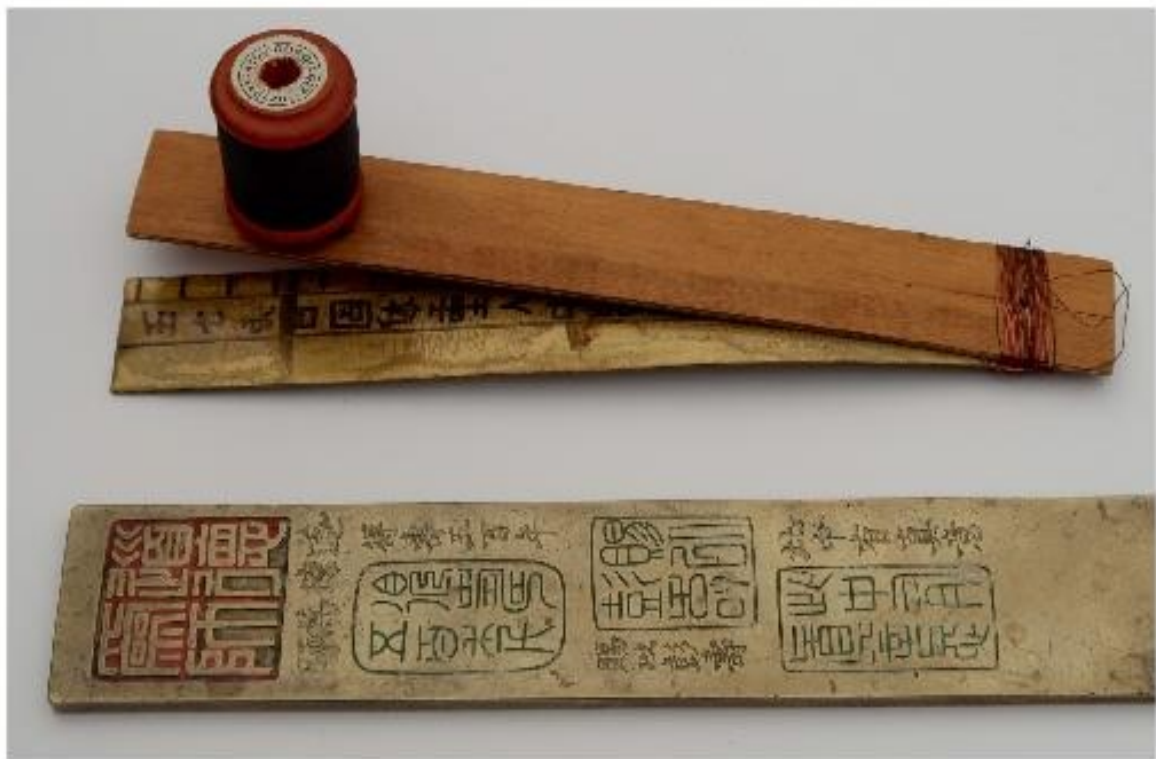
Ursula's homemade Morse code tapper, constructed from a metal ruler, a cotton reel, a strip of wood, and a length of copper wire.
