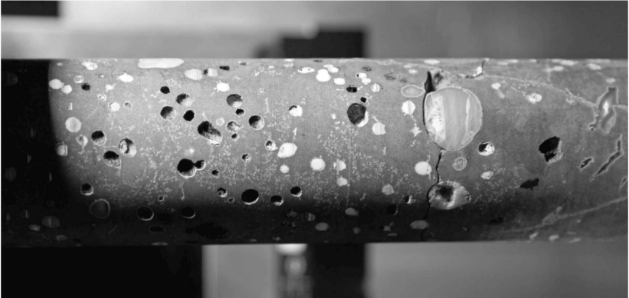
A basalt core with pockets of calcium carbonate
