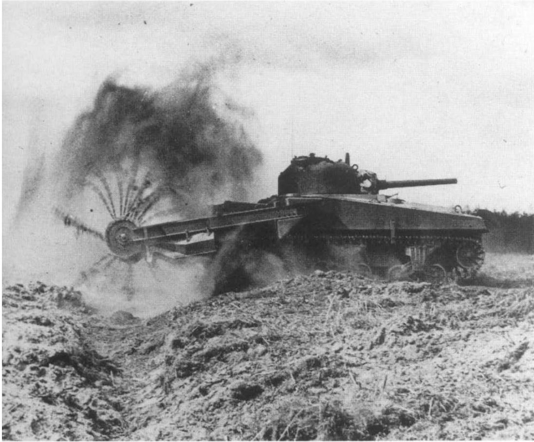
Maj. Gen. Percy Hobart attached all types of gadgets to the British tanks, this one a flail tank. The steel chains thrashing ahead of the rotating drum would set off mines harmlessly. (IMPERIAL WAR MUSEUM)
