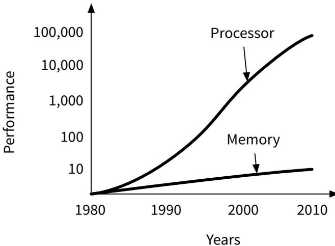
**Figure 7.10** The processor-memory gap in the last decades.
