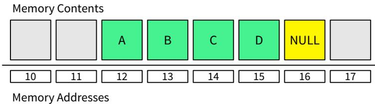
**Figure 4.1** An array in the computer's memory.
