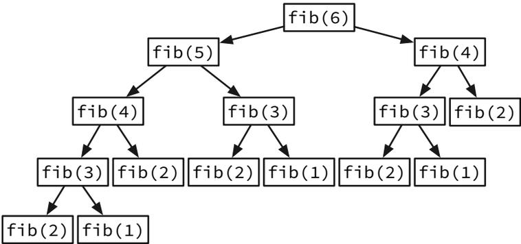
**Figure 3.3** Calculating the 6<sup>th</sup> Fibonacci number recursively.
