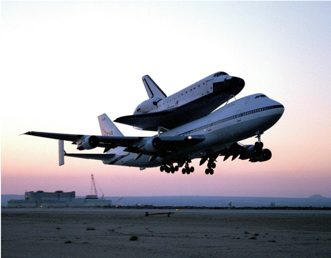
Challenger rode the Shuttle Carrier Aircraft, a customized 747, to Cape Canaveral. (NASA)
