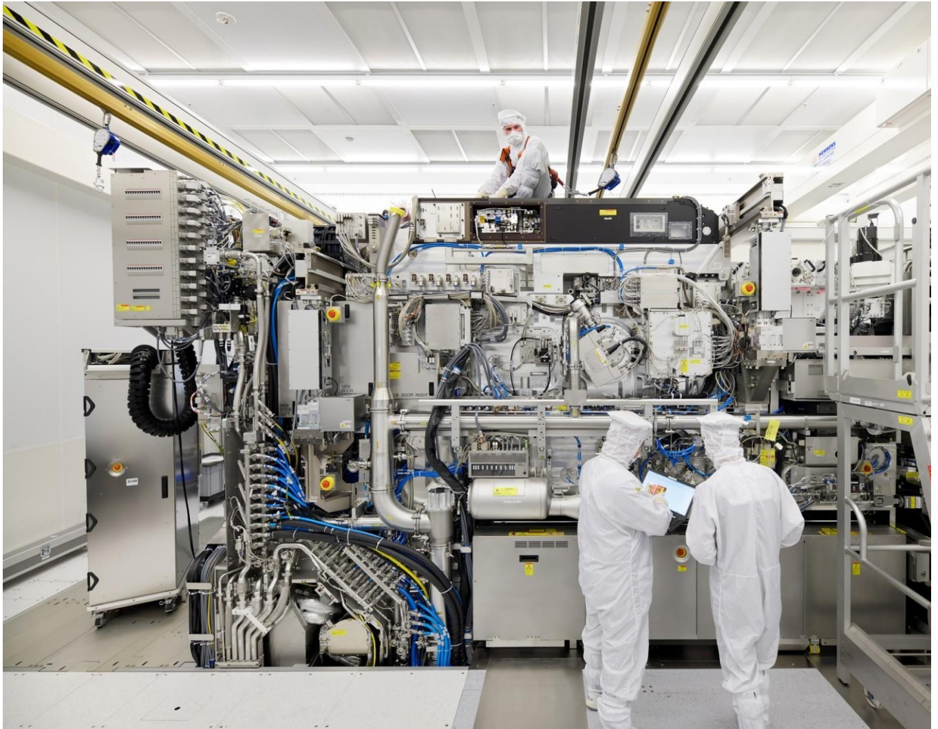
The most advanced lithography machines, which are used to pattern millions of microscopic transistors, each far smaller than a human cell, are made by ASML in the Netherlands. Each machine costs well over $100 million dollars and is built from hundreds of thousands of components. (ASML)
