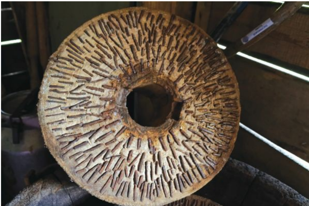
Figure 6.19. Chuvash hand quern wheel with metal staples. Kshaushi, Chuvashia, Russia.
