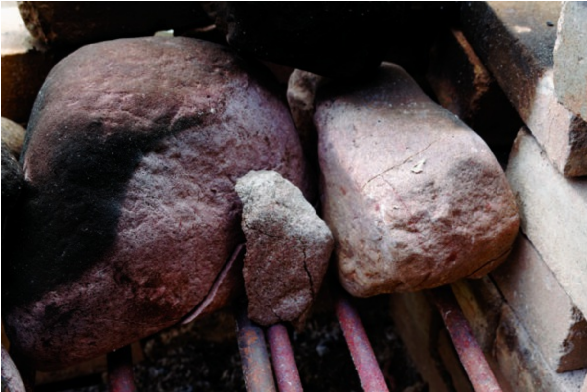
Figure 5.13. Cracked stones. Note the sharp fracture lines from heat shock.
