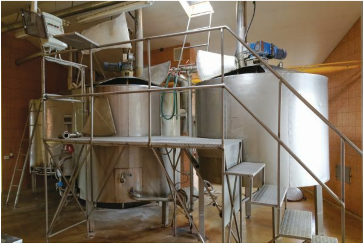
Figure 10.3. The brew kit at the Piniavos brewery. Mash tun on the right, lauter tun to its left.
