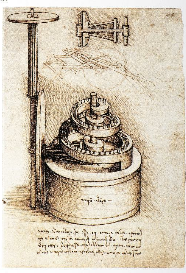
Fig. 53. A spiral gear for equalizing spring power.
