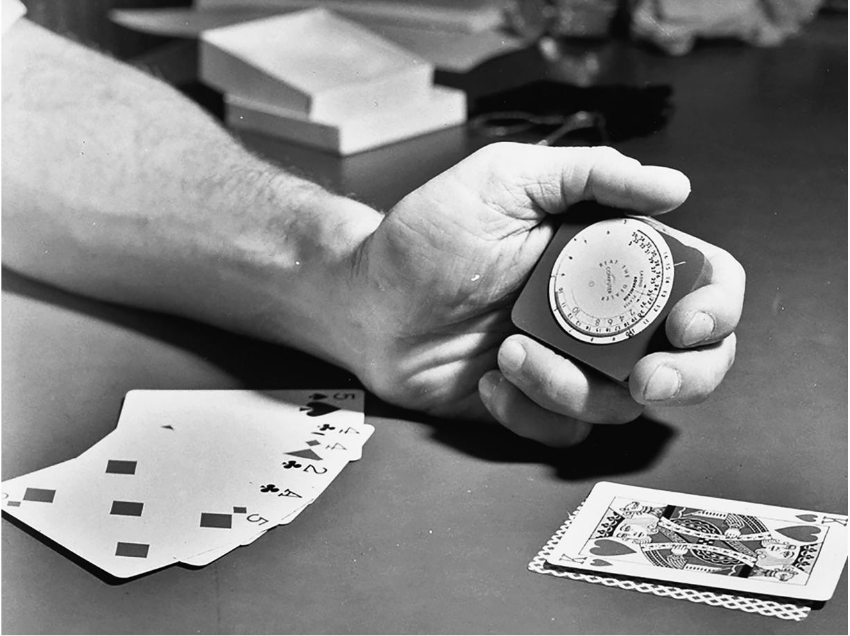
A simple mechanical device for counting cards and calculating the advantage, built in 1964.
