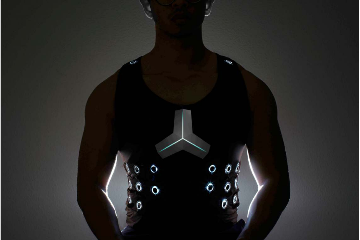
The Neosensory Vest. Sound is translated into patterns of vibration on the skin.
