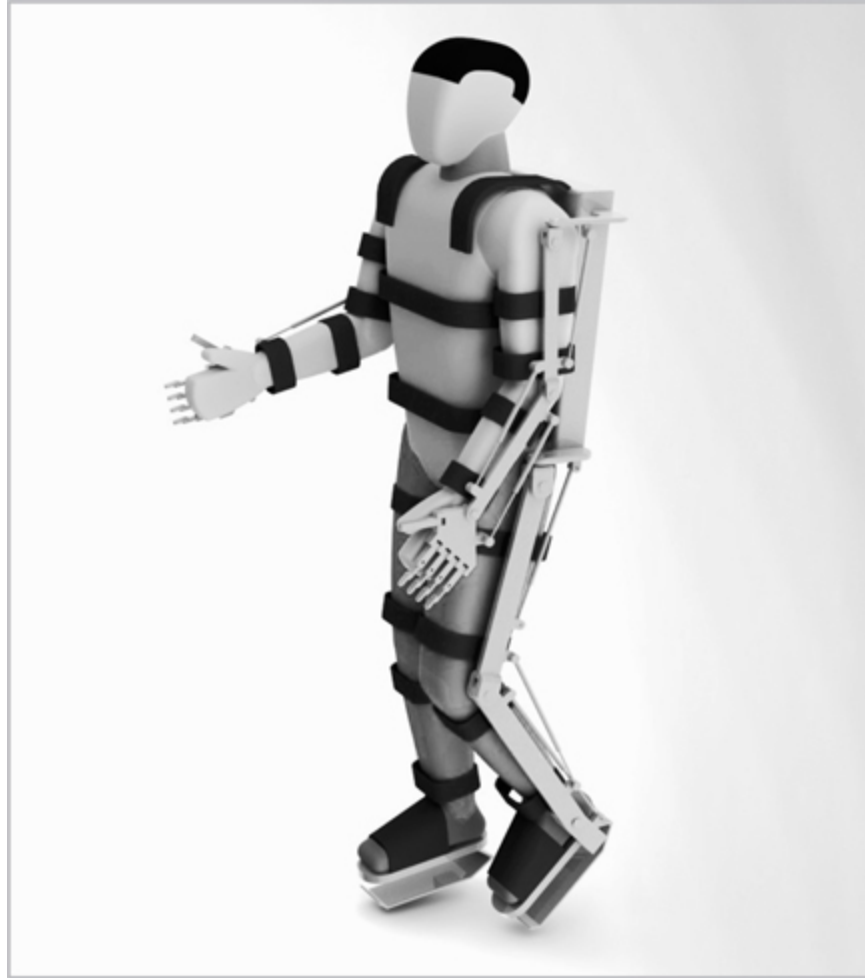
Figure 10. This is the exoskeleton that Dr. Nicolelis hopes will be controlled by the mind of a totally paralyzed person.
